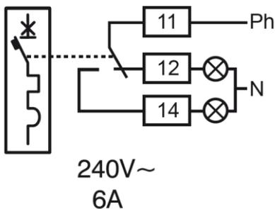
. (terminals marking on the 2<sup>nd</sup> CA are 21 / 22 / 24 when the selector of the reference 406 266 is in the "CA" position).
